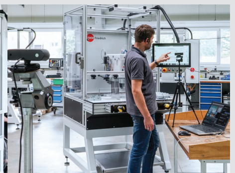
Video acceptance in the factory at FMW before delivery to the customer
