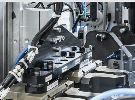
... Tensioning, gripping and clamping units support the assembly processes
