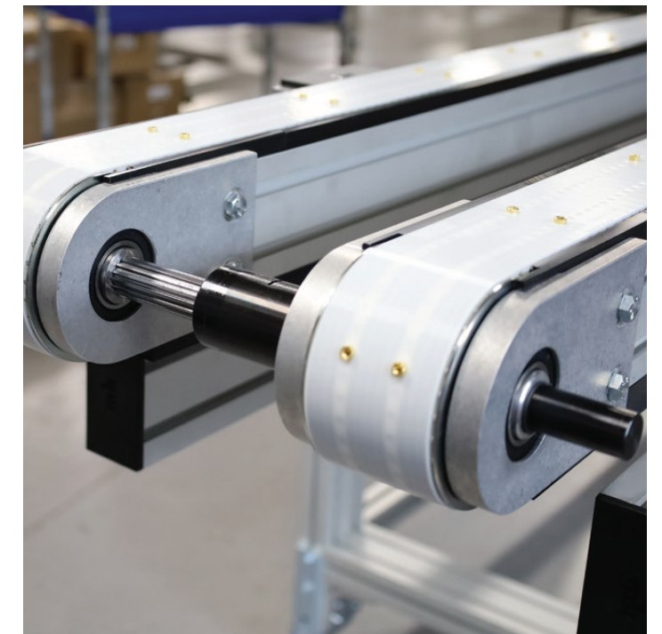
In this example one can see the inserts in the timing belts on this conveyor, as well as the spline shaft used to make the conveyor adjustable in width.
