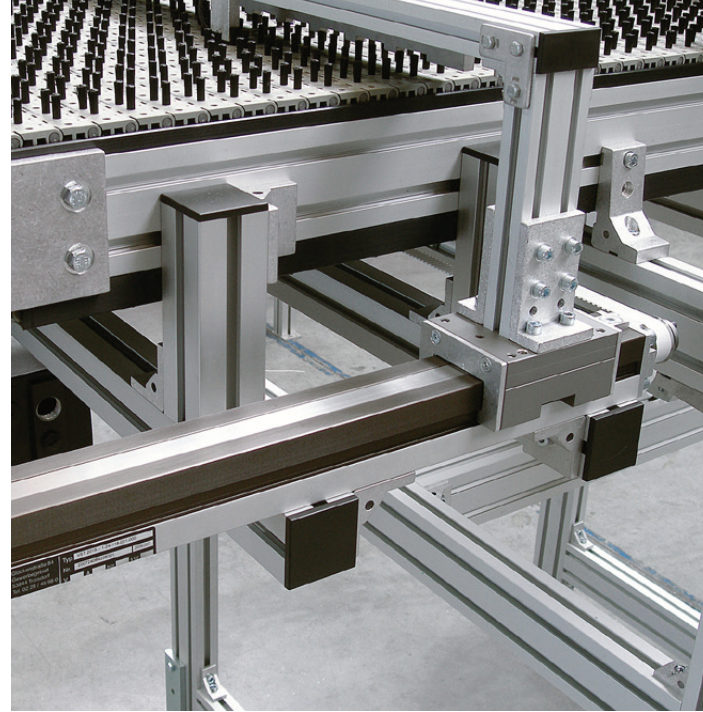
A VST is mounted to the side of the conveyor allowing for tooling to effortlessly be moved across the surface of the conveyor belt.
