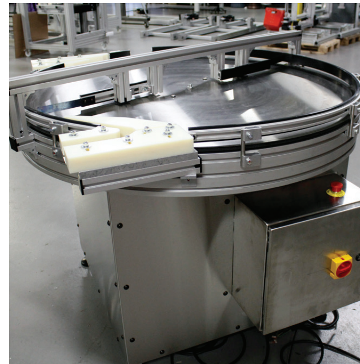
The DTZ-P 2040 Rotary Table is excellent for accumulating product between workstations, or for product overflow.
