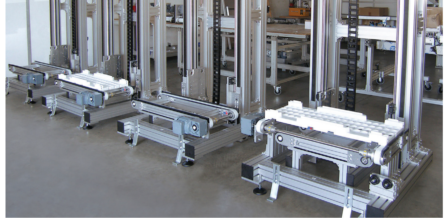
As seen in this example, LZRs are typically used with conveyors to create vertical transfer units, also known as elevators.
