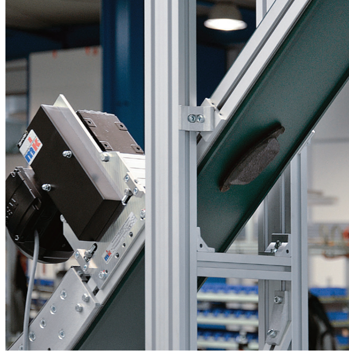
In this example of an engineered solution; a magnetic conveyor carries a metal part on the underside of the belt, up an incline.
