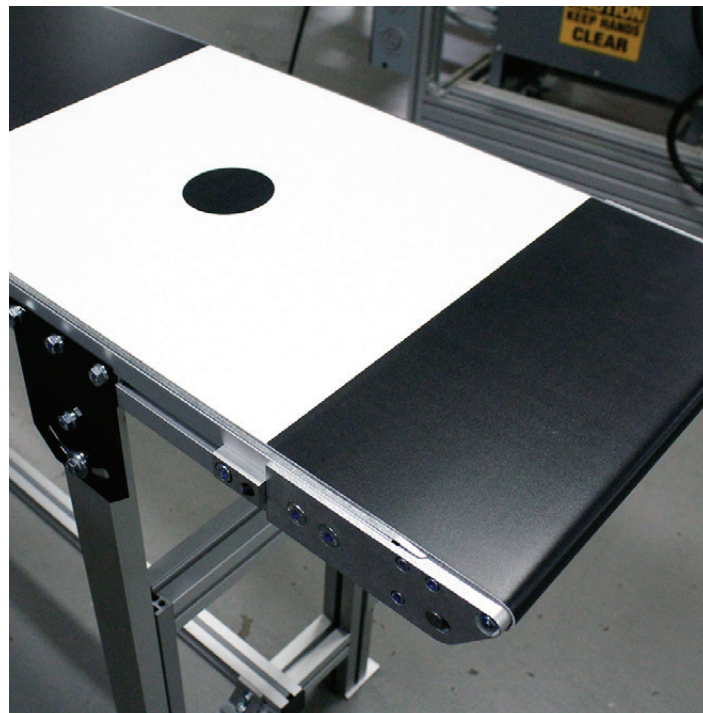
There are nearly limitless belting options available for mk's Belt Conveyors, including belts with custom printed surfaces – such as the one shown above.
