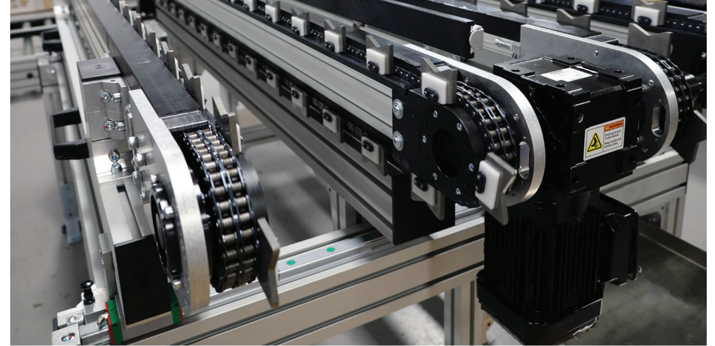
In this example we can see two TKU 2040 units, running parallel, both featuring the optional adjustable width.
