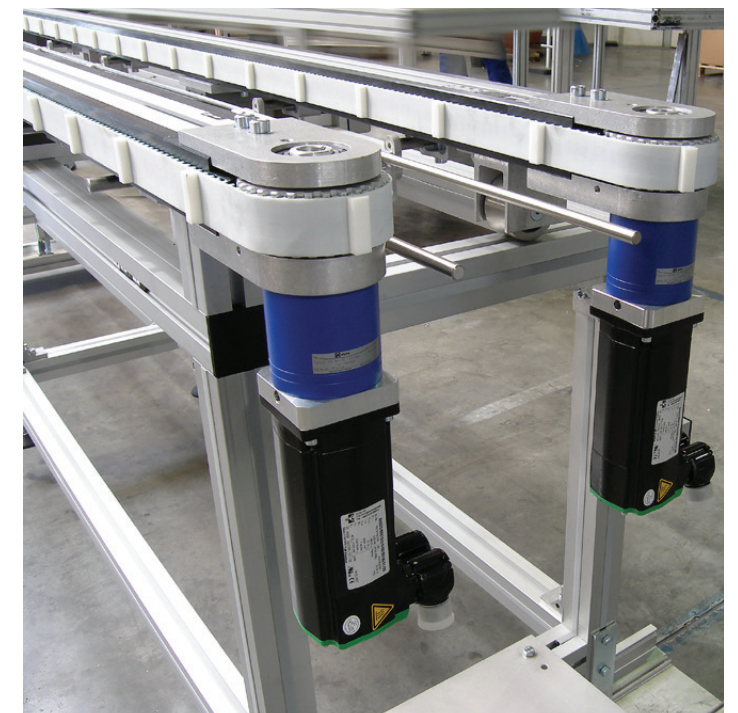
Conveyors can be designed so that they run on their edges. This can be extremely useful when it is necessary to grip products by their sides.
