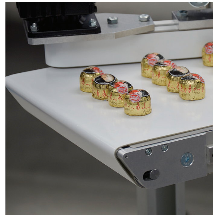
GUF-P 2000 Belt Conveyors have many idler options including a 19 mm rolling nose bar, as shown above.
