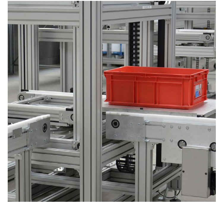
Different modules can be combined to make a single unique module, such as the Right Angle Transfer Unit, mounted within a Vertical Transfer Unit.
