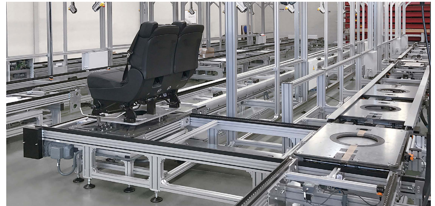
VersaMove pallet-handling conveyors can be designed for product of various sizes – including tall products with an unusual center of gravity.
