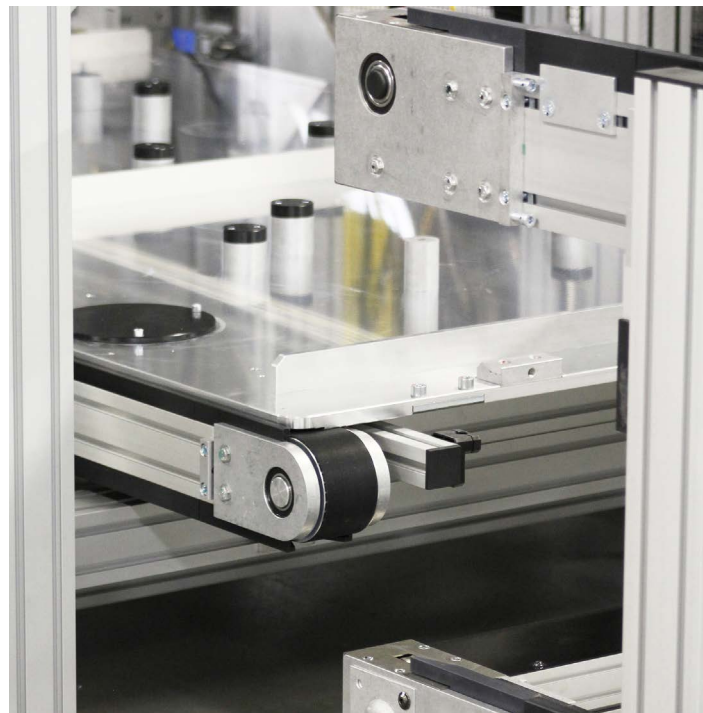
A KHL 2012 Vertical Transfer unit lowers to deliver a pallet to an SRF-P 2012 Accumulating Roller Chain Conveyor.
