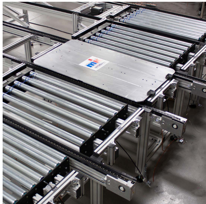
VersaMove Plus conveyor system with SRF-P 2010 main line conveyors, complete with RBM 2010 Lift and Transfer and spur conveyors.
