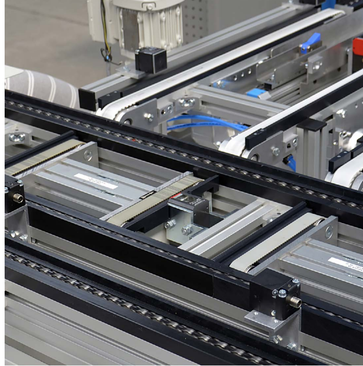
Lift and Transfer Conveyors are typically used to move pallets off the main line and onto spur lines to operators.
