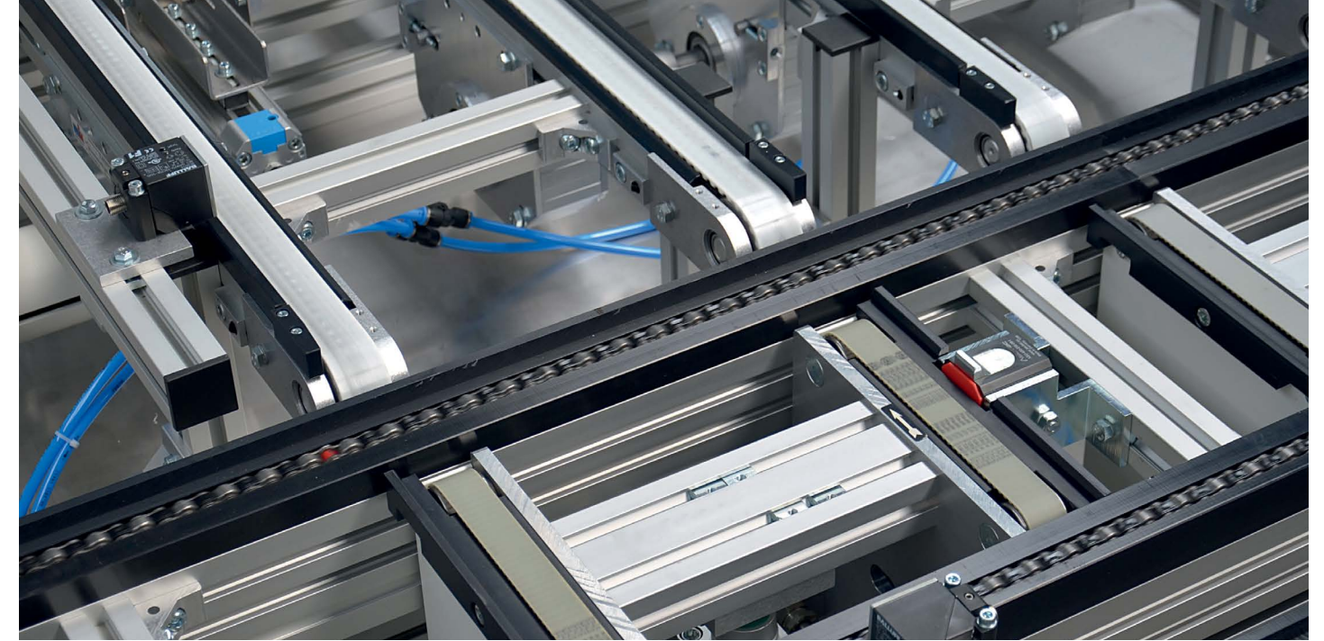
SRF-P 2010 main line Accumulating Roller Chain Conveyors, with ZRF-P 2010 Timing Belt Conveyor, bi-directional spur conveyors.
