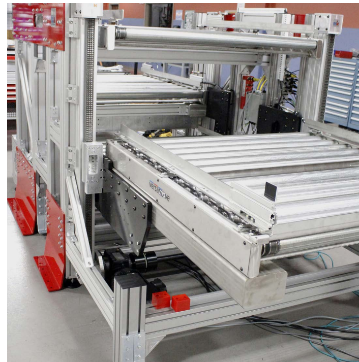
mk is able to accommodate customizations including Vertical Transfer Units featuring Roller Conveyors.
