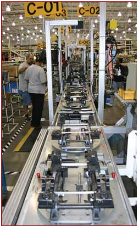
Seats are assembled on a palletized conveyor system. This line assembles second-row rear seats for the Hyundai Santa Fe. Photo courtesy Lear Corp.
