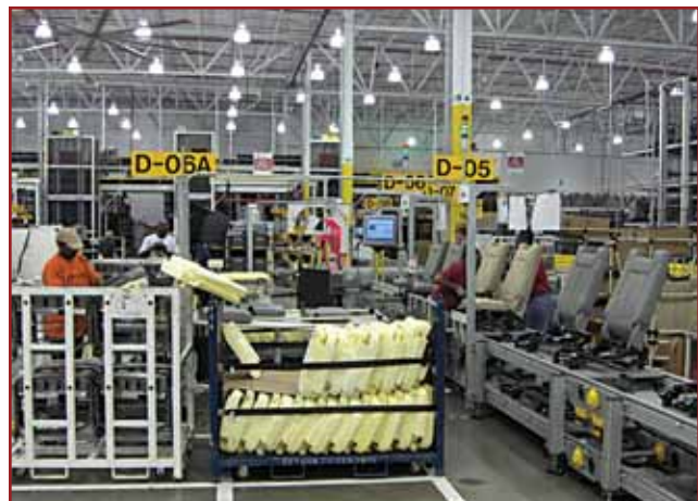
These foam seat bottoms will be covered with fabric trim, then attached to metal frames. Photo by Austin Weber
