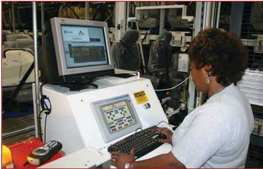
The PC-based interlock system improves overall quality by monitoring the entire seat build process. Photo courtesy Lear Corp.
