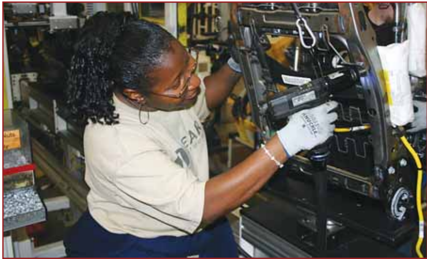
A side-impact airbag is attached to a passenger-side front seat. Photo courtesy Lear Corp.
