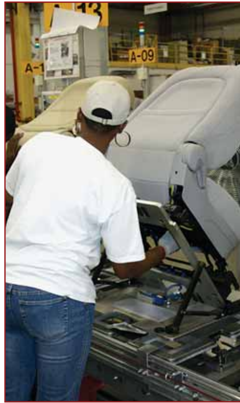
Seats are assembled on pallets that can rotate and tilt for accessibility and flexibility. Photo courtesy Lear Corp.
