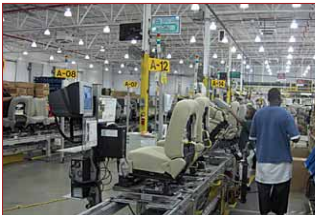
Lear Montgomery assembles more than 300,000 sets of seats annually. This assembly line builds front seats for the Hyundai Sonata sedan and Santa Fe sport utility vehicle. Photo by Austin Weber
