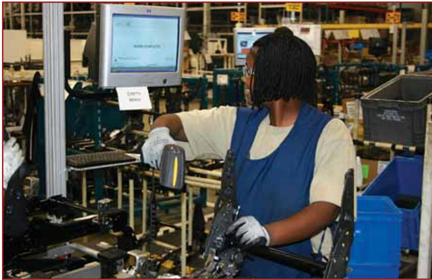
Once a "work complete" message appears on the screen, operators can unclamp the part they're working on and activate the conveyor. Photo courtesy Lear Corp.
