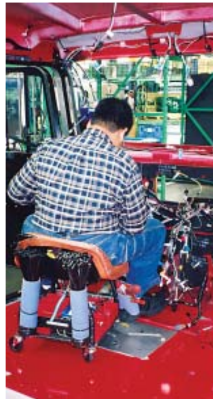
An assembler installs a wiring harness in the cab of a Kenworth truck. Many vehicles are equipped with state-of-the-art tools, such as navigation systems, satellite radio, collision avoidance warning systems, night vision and stability control braking systems, making assembly and testing more complex. Photo by Austin Weber
